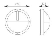
50,000hr maintenance free 20W 3000K 1100lm Fortimo Twist LED Module with integral driver
