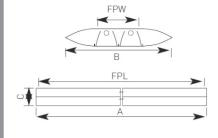
FPL = Fixing Point Length FPW = Fixing Point Width
