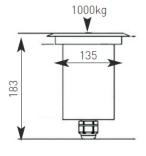
Caution: surface glass temperature will get very hot under normal halogen operation. It is recommended to use GU10 CFL or LED lamps for cooler operation.
